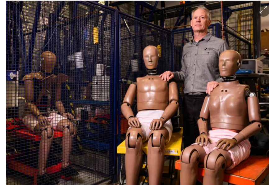
cap’s new female dummy has a female-shaped pelvis and breasts. She weighs 47.5kg, is 1.5m tall and has 150 sensors that will measure the impact of a crash on areas where women are particularly vulnerable. Photograph: James Gourley/The Guardian – March 2024
